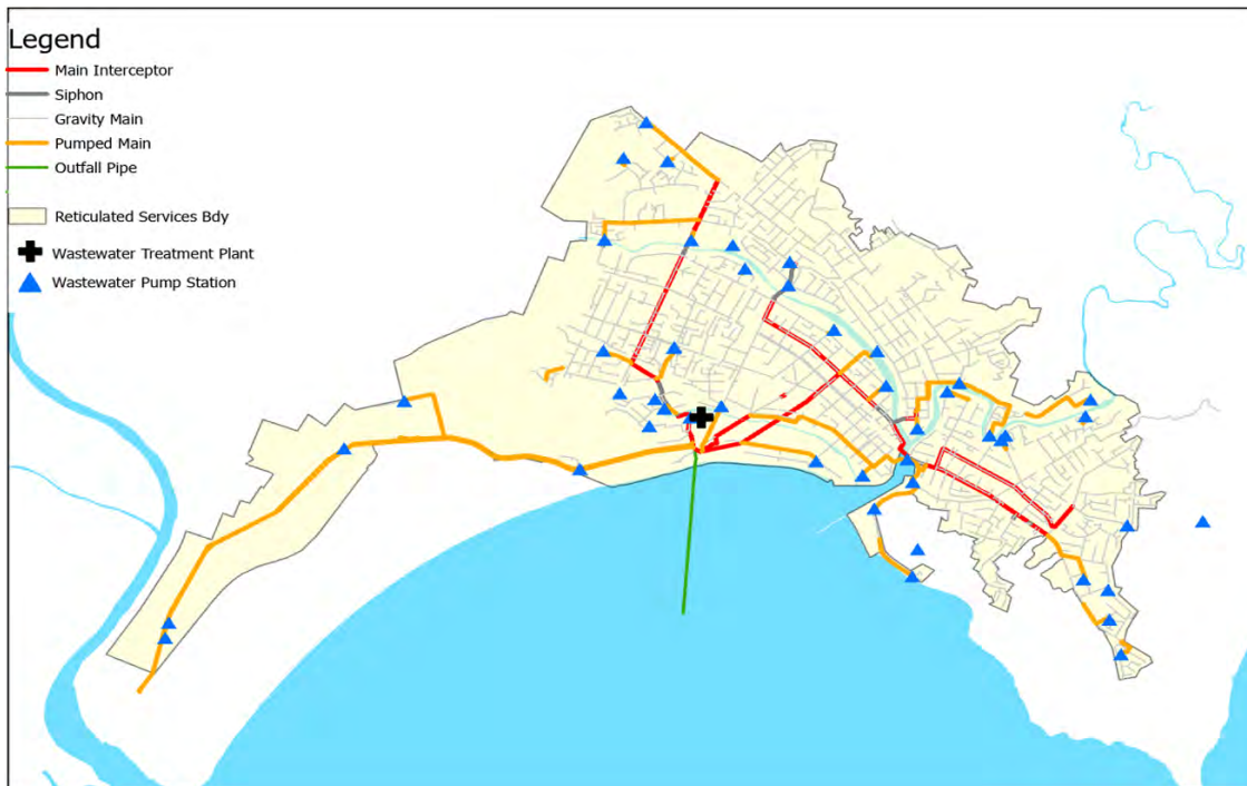
Figure 4: Gisborne city wastewater network
