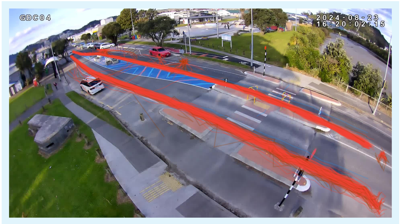
Path tracelines showing the path of motorcycles (blue lines), cars (red lines), and LGVs (brown lines) from 4:20pm - 5:20pm on Friday 23rd August 2024.
