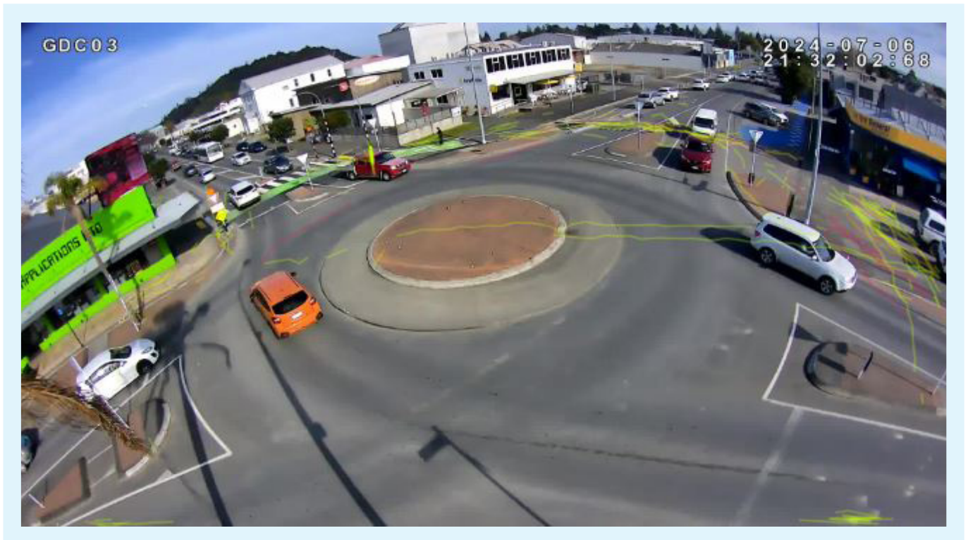
Path tracelines showing the path of pedestrians (yellow lines) and bike riders (pink lines), from 4:30pm - 5:30pm on Friday 23rd August, 2024.
