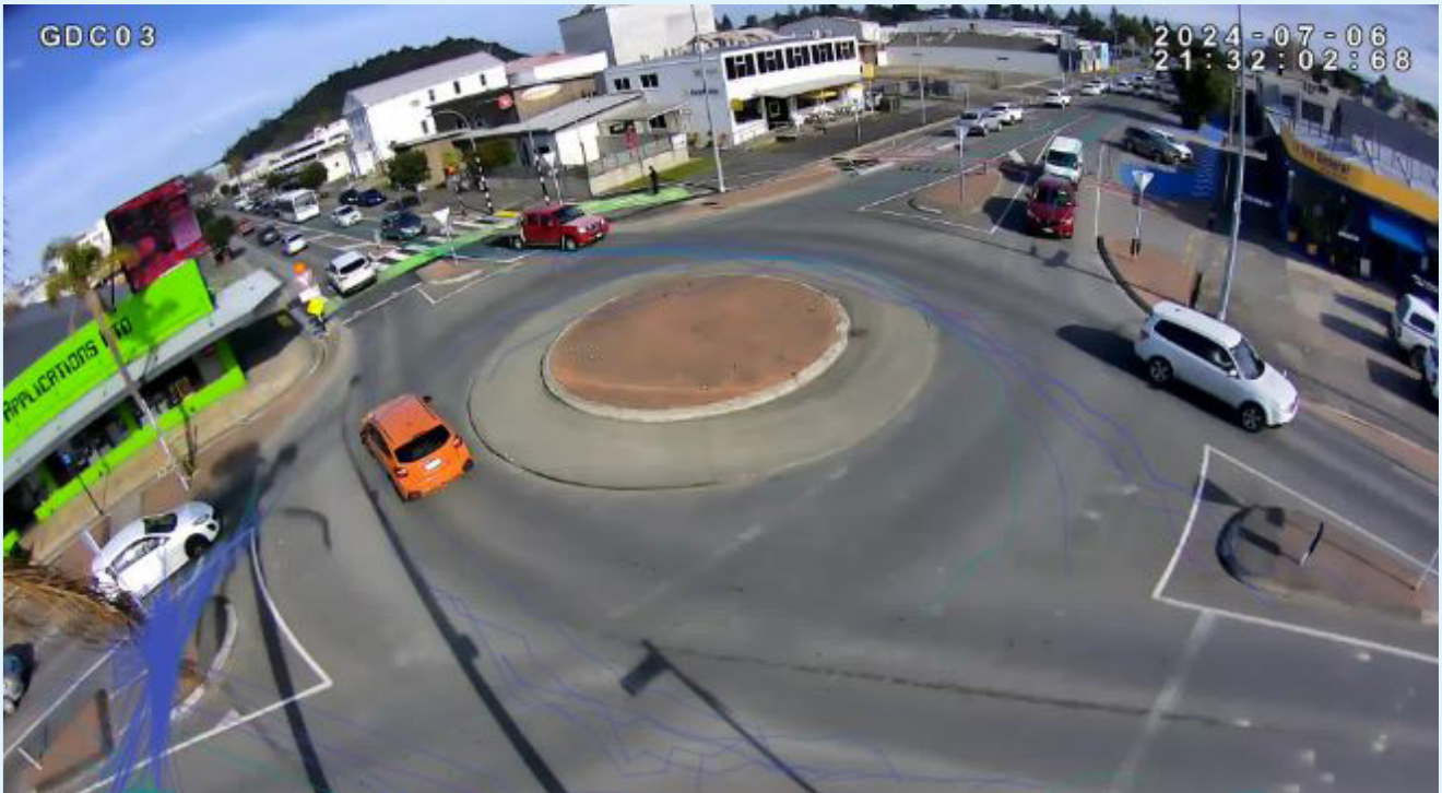
Path tracelines showing the path of buses (blue lines), box trucks (aqua lines), and semi-trailers (purple lines) from 5:30pm - 6:30pm on Friday 23rd August 2024.
