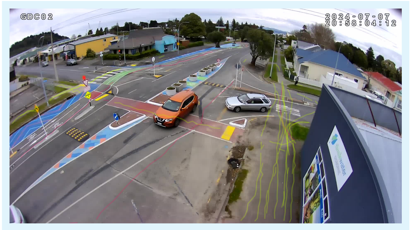
Path tracelines showing the path of pedestrians (yellow lines) and bike riders (pink lines), from 10:00am - 11:00am on Saturday 24th August, 2024.
