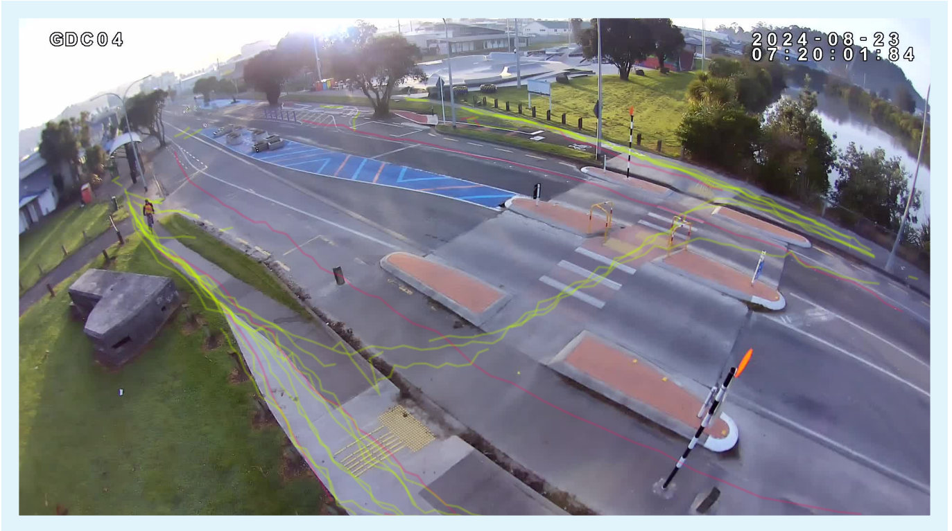
Path tracelines showing the path of pedestrians (yellow lines) and bike riders (pink lines), from 7:20am - 8:20am on Friday 23rd August, 2024.
