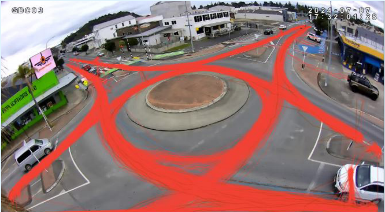
Path tracelines showing the path of motorcycles (blue lines), cars (red lines), and LGVs (brown lines) from 10:30am - 11:30am on Saturday 24th August, 2024.
