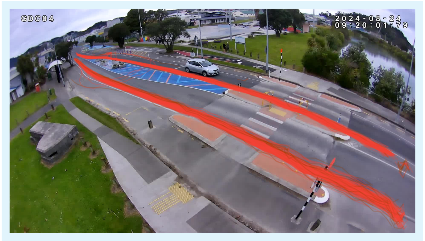
Path tracelines showing the path of motorcycles (blue lines), cars (red lines), and LGVs (brown lines) from 9:20am - 10:20am on Saturday 24th August, 2024.
