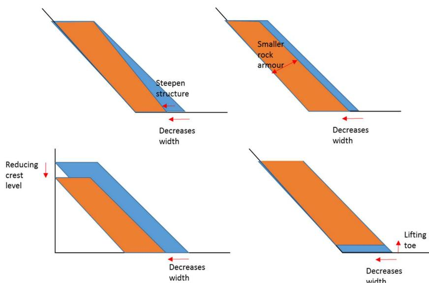
**Figure 3 Typical methods for reducing structure footprint**
