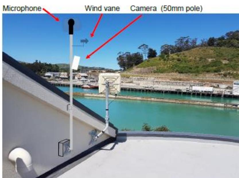
50mm pole with camera, microphone and wind vane. (Not to scale)
