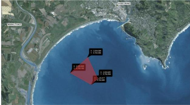
**Offshore Spoil Disposal Ground Plan**
