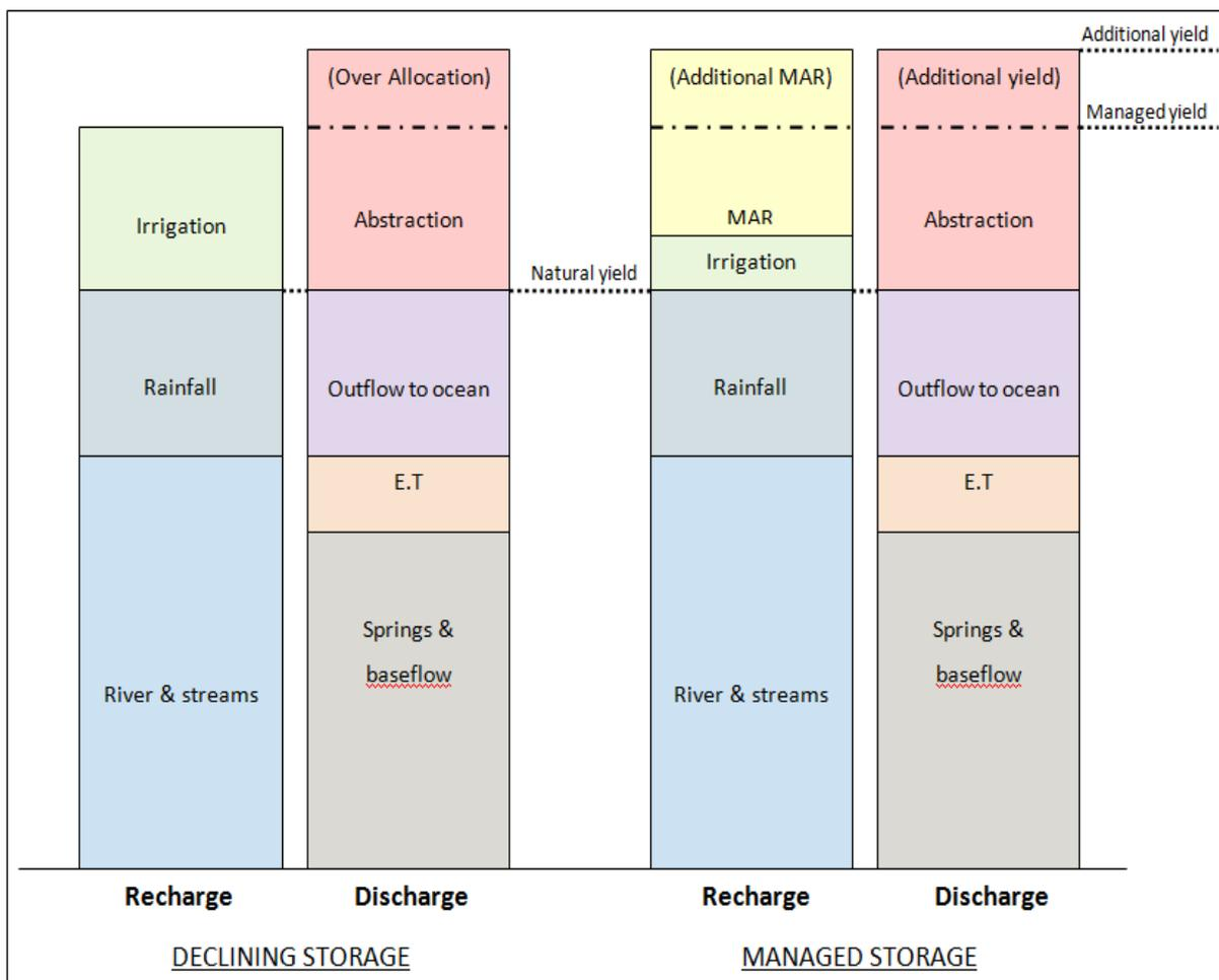
**Figure 2:** Catchment scale water balance and the use of MAR for sustainable and additional yields (Golder Associates, 2013b).
